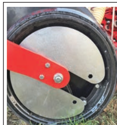
New depth gauge wheel for both open and closed operation depending on soil types etc.
