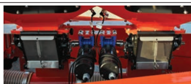
Single shot seed and fertilizer distribution system.
